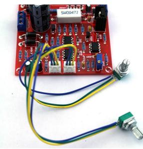
After the installation, please double check that everything is in its place, and then you can start the power and test the device. Please make sure that you have installed cooling fin of considerable size on Q4 (D1047) before starting the power, and the cooling fin should be insulated from the circuit. If the cooling fin is not sizable enough, the cooling fan is thus a must, for which a 24V socket has been kept for this purpose on the
