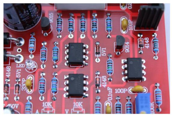
The potentiometer could be placed directly onto PCB, and could also be lined onto the board through its socket and wires. Potentiometer tagged with A is the current limit potentiometer and V is the voltage potentiometer. The voltage potentiometer could be substituted by 10K multi turn wire-wound potentiometer at your own will, with which you could adjust in a more accurate way.
