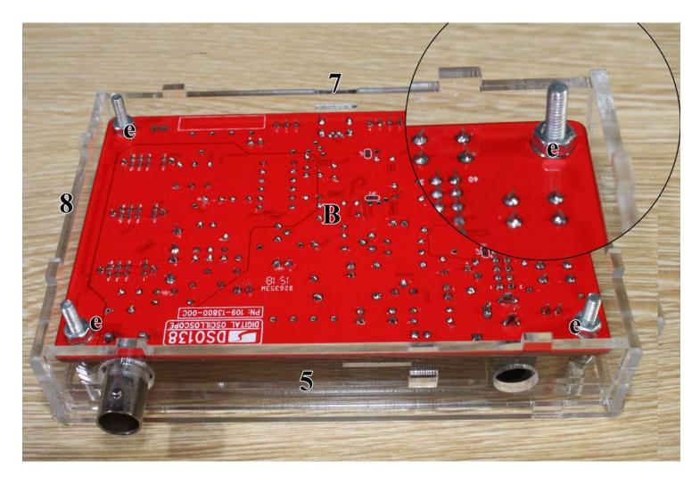
9, Final installation 9 plate, and covered with M3 screws.
