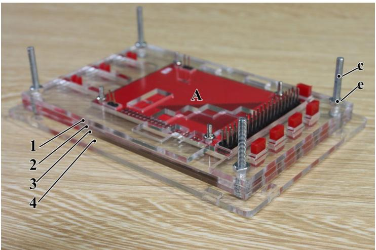
7, Use M3 long screw fixing 1, 2, 3, 4 board, ready to install 5, 6, 7, 8 plate.
