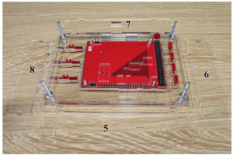
8, Plug in the oscilloscope motherboard and LCD, while the red button and the button on the motherboard are aligned and mounted on the motherboard plate numbers 5,6,7,8. Fixed with the M3 screws.
