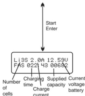
If both numbers are identical you can start charging process. If not, press BATT TYPE/ STOP button to go back to previous screen to recheck the number of cells of the battery pack before going ahead.
