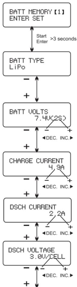
For your convenience UP100AC DUO has a data storage and load program, it can store 10 different battery data represent the respective specifications of batteries, you can call back the data when charging/discharging without setting up the program again, press START/ENTER button to make it blink and use INC. or DEC. to set up the parameter.
