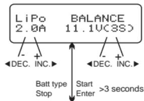
The left side of the first line shows the type of battery you choose. The value on the left of the second line of the charger is current the user sets. After setting the current and voltage, press the START/ENTER button for more than 3 seconds to start the process.
