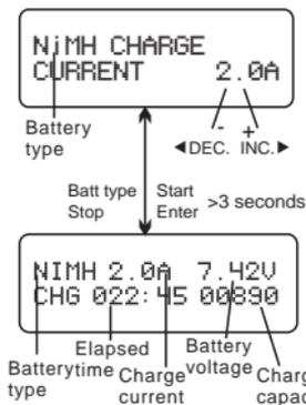
This program is for charging and discharging of NiMH/NiCD batteries associated with R/C models applications. You can press Inc. or Dec. button to change the parameter value, press START/ENTER button to store the value.
