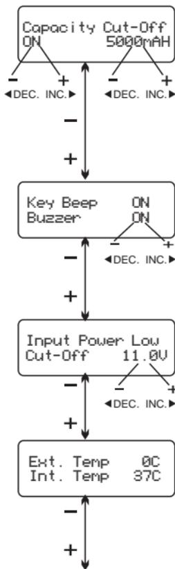
This program sets the maximum charge capacity that will be supplied to the battery during charge. If the deltapack voltage is not detected nor the safety time expired by any reason, this feature will automatically stop the process at the selected capacity value.
