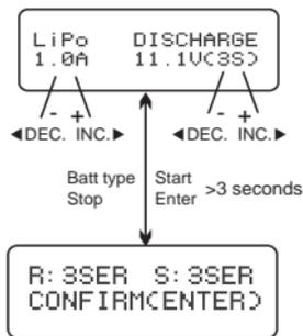
The value of discharge current on the left can not exceed 1C, and the value on the right can not be under the voltage recommended by the manufacturer to avoid over discharging. press the START/ENTER button for more than 3 seconds to start discharging.
