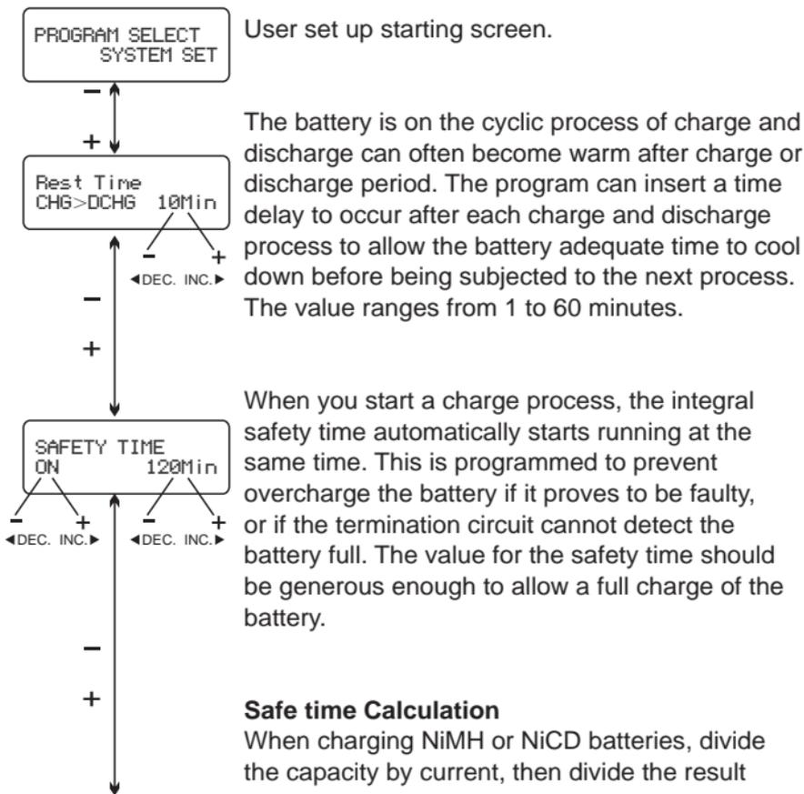
by 11.9, set this number as the value for safety time setting. If the charger stopped at this threshold, about 140% of the capacity will have been fed into the battery.
