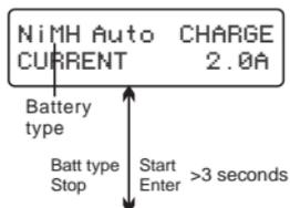
The program is for charging of NiMH/NiCD batteries in auto mode.
