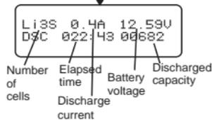
This screen shows the real-time status of discharging, you can press BATT TYPE/STOP button to stop discharging.
