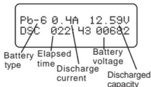
The screen display the real-time discharging status. Press START/ENTER button to change the discharging value. Press START/ ENTER button again to store the parameter value you set. Press BATT TYPE/STOP button to end the program.
