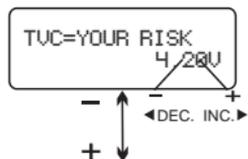
Set the terminal voltage, it can be adjusted (4.18-4.30V)
