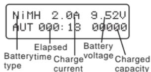
The screen displays real-time charging status. Press BATT TYPE/STOP button to stop the process.
