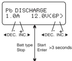
Set up the discharge current on the left and nominal voltage on the right. Range of discharge current is 0.1-5.0A(CH1), 0.1-2.0A(CH2), the voltage should match the battery being discharged. Press ENTER/START button for more than 3 seconds to start discharging.
