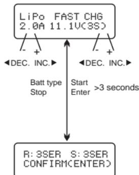
The value on the left side of the second lines shows the charge current. The value on the right side of the second lines shows the battery pack's voltage. After setting current and voltage, press the START/ENTER button for more than 3 seconds to start the process.
