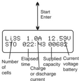
This screen shows the real-time status charging. Press BATT TYPE/STOP button once to stop the charge process.
