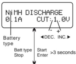
Set discharge current on the left and final voltage on the right.
