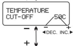
Set the cut-off temperature, it can be adjusted(20°C/68°F-80°C/176°F).
