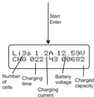
If both numbers are identical you can start charging process. If not, press BATT TYPE/ STOP button to go back to previous screen to recheck the number of cells of the battery pack before going ahead.
