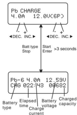
Set up the charge current on the left and nominal voltage on the right. Range of current 0.1-10.0A(CH1), 0.1-6.0A(CH2), the voltage should match the battery being charged. Press START/ENTER button for more than 3 seconds to start charging.
