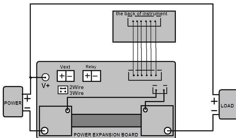
Two wire system wiring diagram
