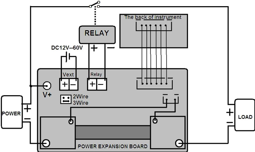
According to connection diagram method to connect the wire , connection instrument and power expansion board with 6 p ribbon cable, jumper cap should be pick up on the 2 wire, the upper left corner of the power expansion board is V + ,this V+ and the positive of load should be connect with the positive pole of power ,the cathode of the power should be
