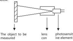
It must be ensured that the object to be measured is fully within the field of vision afforded by the temperature measurement meter, that is, the meter can see nothing but the object to be measured. The greater the object to be measured is, the farther the distance detected by the meter may be. The smaller
