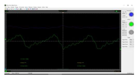
Don't worry too much about the waveforms at this stage a large amount of the "distortion" is due to the fact that the mixer is not actually mixing two proper signals the output from M1 is going to be from the "airborne" and "PSU" 50Hz mains. The main thing is they are both 8MHz showing the mixer is working.
