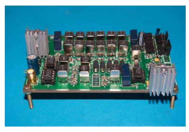
This is an idea to make your boards easier to handle when soldering use nuts and bolts to make temp legs to keep the board level and stable when soldering. This was my first "practice board" I still have to fault find and get this one working. It was also my first attempt at SMT!
