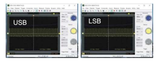
I had problems with the oscillator at this point all I can say is it was one of two things either a sub-standard socket or my scope was somehow loading the oscillator part of the circuit (TP18) and I could only get it to ossel on three of the four modes. To solve this I replaced the socket and I also shifted TP18 from pin 6 to pin 7 to minimise loading. Problem solved.
