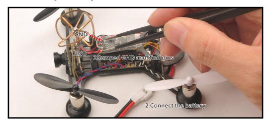
2.Select RX setup to AFHDS Mode, turn on the transmitter while holding the bind button
