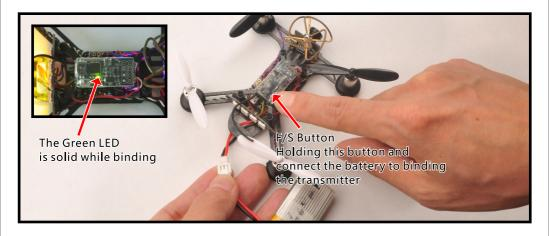
3.Go to the Receiver [Bind] option, and ENT to Bind with the receiver, The transmitter beeps.
