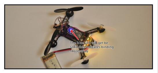
4.Reconnect the Qx95 and the transmitter, the blue LED on the receiver blinking fast again, this indicates Receiver and Transmitter are all works.
