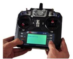
2.Turn on the transmitter while holding the bind button
