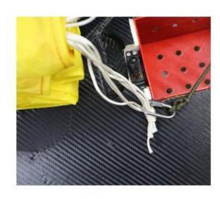
Attach the rope to the umbrella clasp of the fuselage
