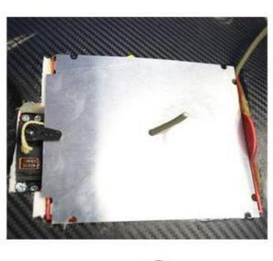
Close the umbrella hatch cover Use a servo to lock the hatch
