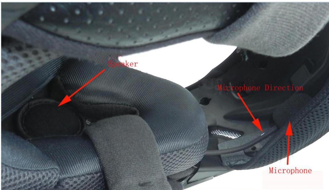
**Note: Please pay attention to the site of the microphone to ensure crystal voice, the white dot on the microphone support should be exactly opposite to the mouth and the distance between the microphone and mouth should be no more than 2cm, improper installation may led to low voice or even no voice.**
