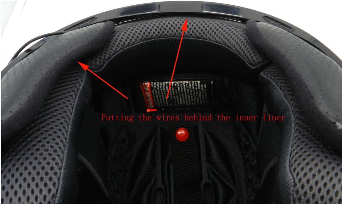
Putting the wires behind the inner liner
