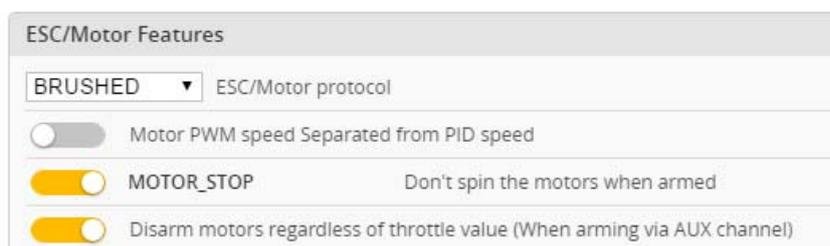
\*This step is in order to avoid motor auto-spinning when connect the battery
