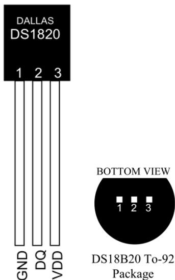
When enter to this function, the Row 2 of the LCD is show a string "1=GND 2=DQ 3=VDD" , it's mean TP1 of the tester connect the GND of the DS18B20 , and so on. The Tester can not sense the pin distribution of the DS18B20, because DS18B20 is a integrated circuit. Must according to the string to install the DS18B20.
