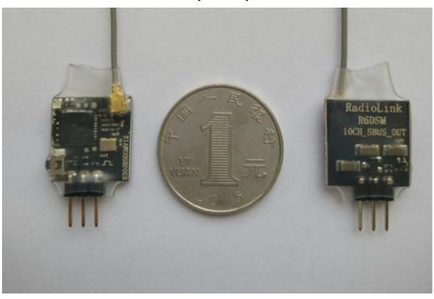
Radiolink R6DSM, 2.4G 10 channels receiver, DSSS and FHSS spread spectrum working synchronously, 1 gram weight, SBUS and PPM signal support, use for Radiolink transmitters AT9, AT9S, AT10 and AT10II, is the best choice for racing drone.
