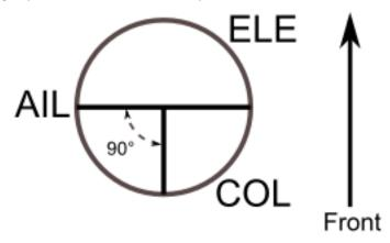
90 (3 Servo): With Aileron input, the aileron and pitch servos tilt the swash-plate left and right; with elevator input, the servos tilt the swash-plate fore and aft; with Pitch input, all three servos raise the swash-plate up and down. Most commonly used for electronic helicopters.
