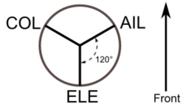
120 (3 Servo): Servos are placed around the swash-plate at 120° intervals. With Aileron input, the aileron and pitch servos tilt the swash-plate left and right; with Elevator input, the three servos tilt the swash-plate fore and aft; with Pitch input, all three servos raise the swash-plate up and down. Servos working in unison dramatically increases the torque available as well as the precision and centering.
