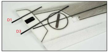
3.2 Install the servo arm,paste the servo into the preserved slot on the wing,and bury the servo wires inside the notch of the wing.
