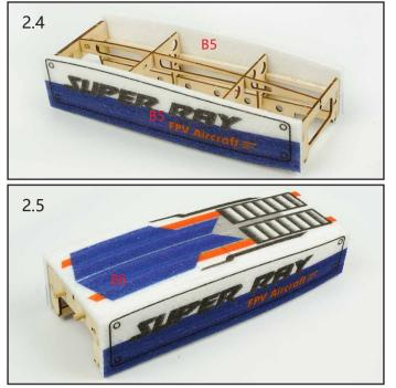
Finish the fuselage assembly, the cabin cover is detachable, and can be locked by latch at the tail.
