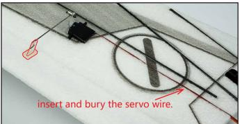
3.4 Insert the servo wire of the wing through the fuselage, and plug the wing onto the fuselage.
