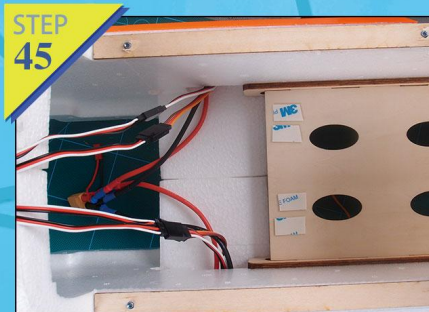
Fig.45-46: The throttle connects white wire, servo signal wire connects yellow wire, yellow wire connects aileron servo, white connects ESC signal, use Y wires to connect two yellow wires and use Y wire is paralleled with throttle, then take out UBEC from power.
