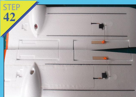
Fig.41-42: Use allocated screws to fix servo horn and pulling rod. The same way to install on both side of wings.
