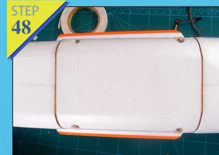
Fig.47-48: Use 4 screws (3mm*30mm) to fix camera canopy.
