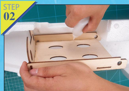
Fig.1-2: Assemble plywood of flight controller cabin and fix it by glue.
