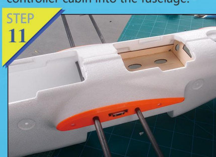
Fig.11-12: Insert carbon fiber tube into fuselage, after air-dry for a while, drag the tube out from the fuselage.
