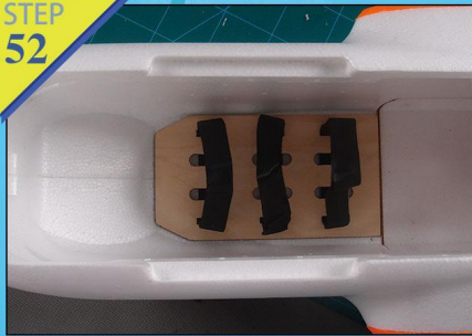
Fig.51-52:Daub the glue on the battery replacement plywood and reserved position respectively, and then joint them together after 2min .
