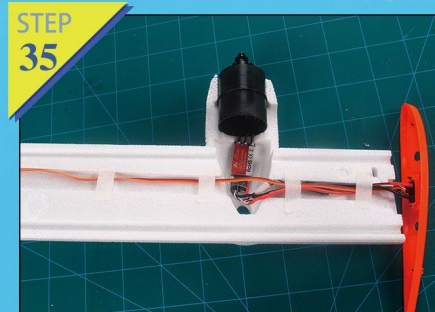
Fig.35-36:Daub the other side of motor protector shell by glue and bond wings together(Attention: align the sideline with motor protector shell and foam. You need to adjust according to the real situation).
