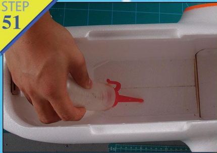
Fig.51-52:Daub the glue on the battery replacement plywood and reserved position respectively, and then joint them together after 2min .
