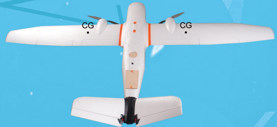
CG: From wingsleading edge to backward 110-115mm
