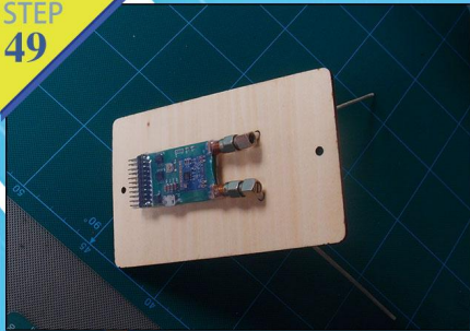
Fig.49-50:Adhere receiver to the plywood and fix the plywood by screws.
