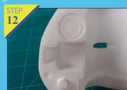
Fig.11-12: Insert carbon fiber tube into fuselage, after air-dry for a while, drag the tube out from the fuselage.
