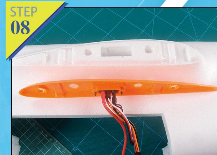
Fig.7-8: Make sure all wires of the connector are right, glue its surface and air-dry for about 2min.
