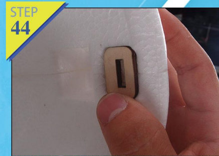
Fig.43-44: Glue the pin fixed plate (install the wood piece according to the reserved position).
