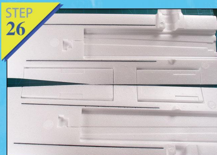
Fig.25-26:Apply glue on the carbon plate, use a cloth to cleanse unnecessary glue when inserting into slot.
