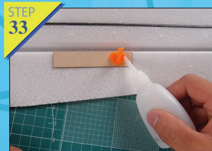
Fig.33-34:Daub glue on the clip to fix servo horn, and adhere glue to the slot of wings(Attention:Glue corner of slot to make sure it is better to glue well).
