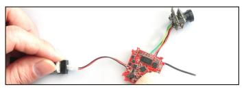
2. Turn on your Frsky Taranis transmitter, and move to BIND OPTION from SETUP MENU, Choose receiver mode D16 or D8 according to your Betaflight receiver configuration (Frsky\_X = D16, Frsky\_D = D8)
