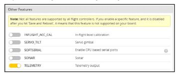
2.After binding successful, turn on the Frsky Transmitter and move to option TELEMETRY, then click "Discover new sensors"
