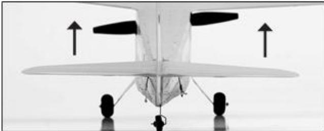
Move the rudder stick left and right to check turn control. When the stick is pushed to the right, the rudder should also move to the right.
