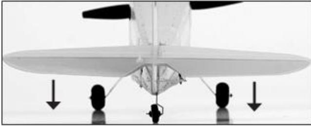
When the elevator stick is moved backward, the elevator should move up. This will cause the nose of the airplane to lift in flight.
