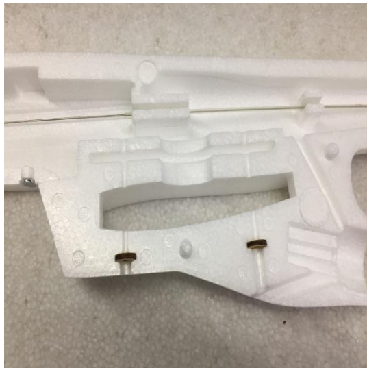
Wood glued to the fuselage
