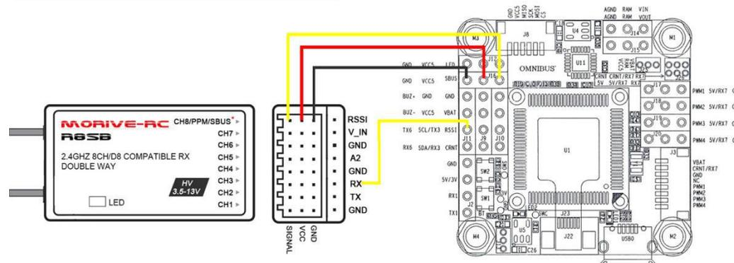
In the GUI PORTS tab, select the UART that corresponds to the receiver (usually UART2 in F7 flight controllers) and activate Serial RX.
