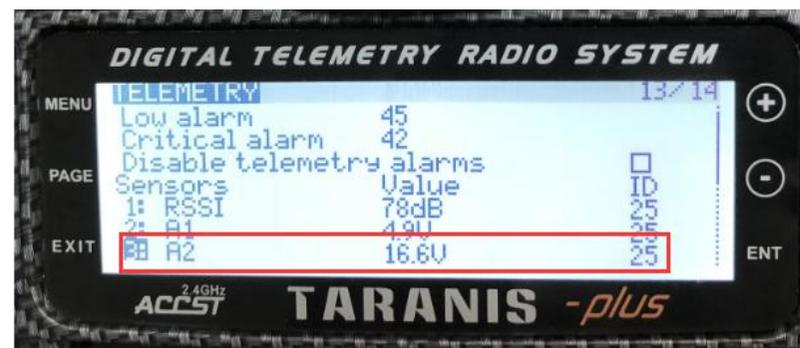
We need to setup the A2 Ratio. Select A2, long press the ENT button to enter the setting interface.
