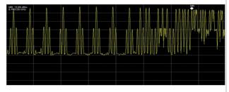
5362—5945M Hz The transmitting power of the 48 channels is almost the same, reaching the standard completely
