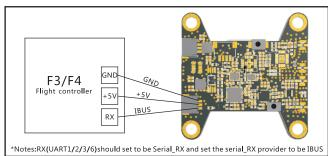
Connect UX14 Receiver to your F3/F4 flight controller. Enable Serial RX for UART1(F4 FC) or UART3(F3 FC), then choose Serial\_based receiver from the Receiver Mode tab, and set the Serial Receiver Provider to IBUS Mode in Betaflight Configurator. The UART Seria rx port please according to the flight controller connection diagram
