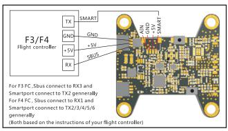
1.Connect UX14 Receiver to your F3/F4 flight controller. Enable Serial RX for UART1(F4 FC) or UART3(F3 FC), then choose Serial\_based receiver from the Receiver Mode tab, and set the Serial Receiver Provider to SBUS Mode in Betaflight Configurator. The UART Seriarx port please according to the flight controller connection diagram
