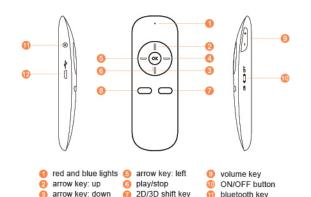
Shift the ON/OFF button to ON to start up.
