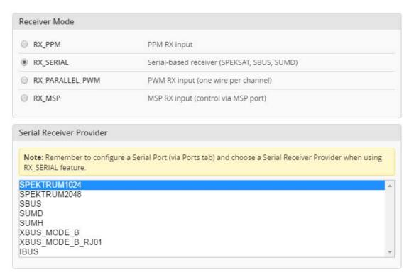
2. SBUS receiver welded to the UART2 GND, + 5V, RX2. Then Enable Seria\_RX and Set Receiver mode RX\_SERIAL, Select Sbus signal in Cleanflight configurator.
