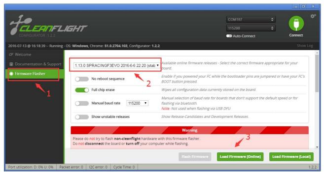
Click "Flash Firmware" and wait the ST DFU DRIVER Automatic installation. It's successfully installed when you see the DFU port on the Up right corner.
