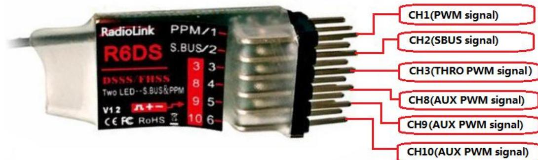
SBUS&PPM output working mode:
