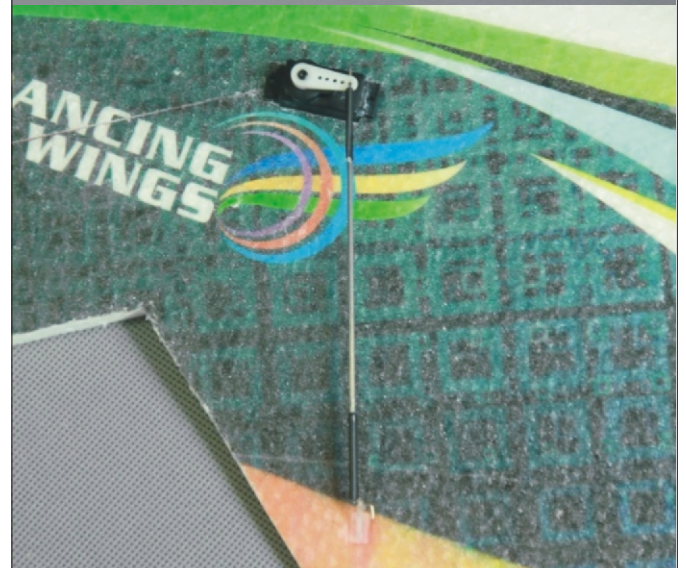
0.03 Make a connecting rod by using the Z-type steel wire and carbon rod, and then connect the servo and aileron.
