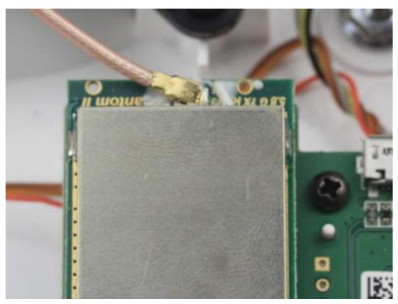
This step is to install the remote control connections need to take down the original antenna, remove the antenna, be careful not to damage to the IPX, remove fixed glue first, and then gently remove the antenna. Then put the connection line (the longer one) connect the IPX, then cover on.
