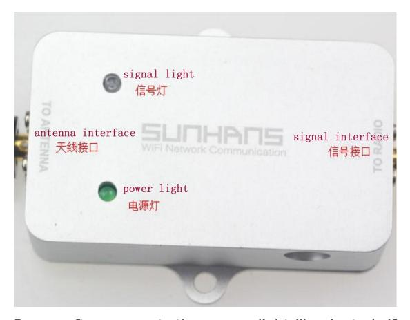
Power after connect, the power light illuminated, if the remote control is open the signal light will bright, if the light is not illuminated, said there was no signal, need to check the reason, before turning on the power supply, please ensure the antenna interface has any antenna installation, otherwise easy to burn out the power amplifier, 2.4 G power amplifier as same as shown above (电源接通后电源灯会亮,如果遥控器开启,信号灯会亮,如果信号灯没亮则表示没有信号,需要检查原因,接通电源前,请先保证天线接口有安装任意一款天线,否则容易烧坏功放, 2.4G 功放也是一样如上图)
