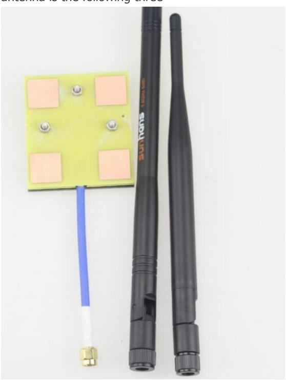
From left to right in turn is a directional antenna, power amplifier with omni-directional antenna, omni-directional antenna
