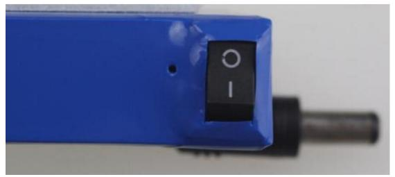
O is turn off, | is open(there have a red light on the left ,the left light have no bright if the battery have no any electricity)
