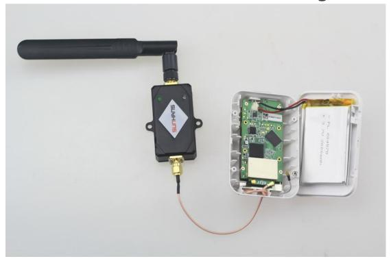
Here to install just pull out the original antenna (pull out the antenna on the right side, left don't move), and then connect the SMA wire inserted into the wireless bridge, fixed the can. This step needs to be punched
